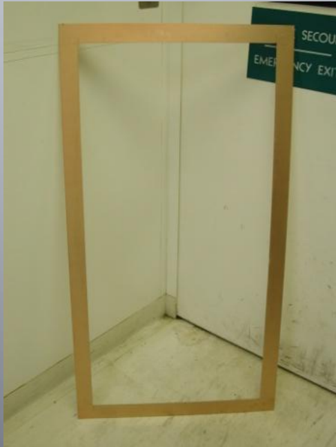
FR4 frame Copper on both sides Electrically isolated
