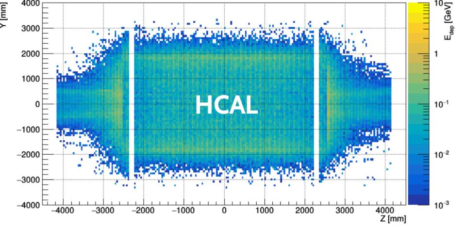
**Energy deposition in calorimeters per bunch crossing**
