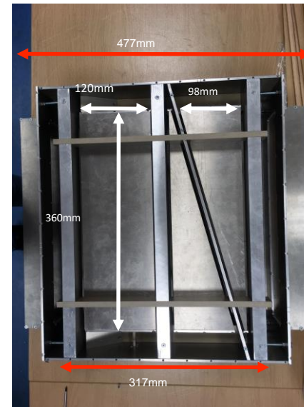
Half-size prototype BPM, tested in the diagnostics lab.
