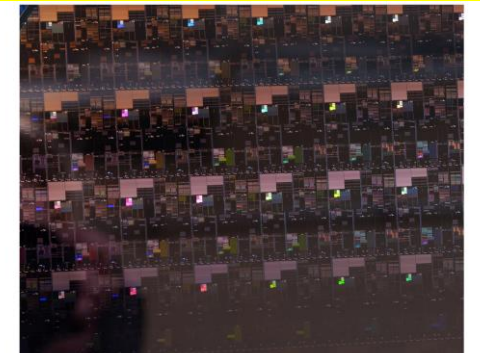
IBM Research 2 nm A close-up of a 2 nm wafer fabricated at IBM Research's Albany facility, with individual chips visible to the naked eye. Courtesy of IBM
