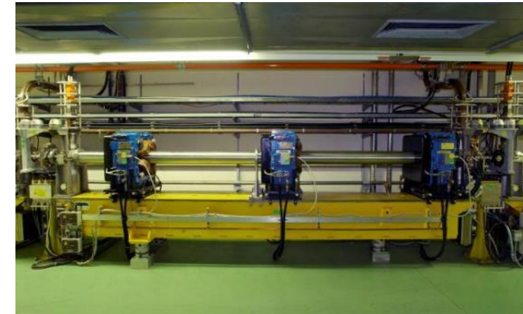
A 3 GHz accelerating structure, 4.5 meters long, energy gain 45 MeV.
