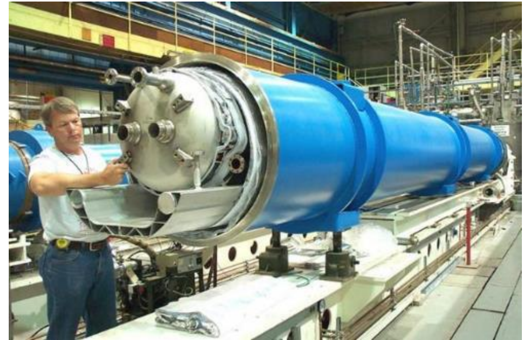
The 1232 LHC magnets contain two pipes, one for each of the counterrotating beams.
