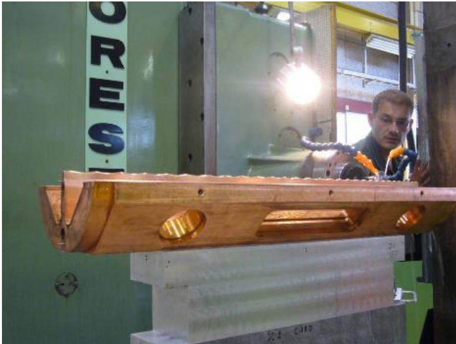
Machining of a vane for the new CERN RFQ (linac4)
