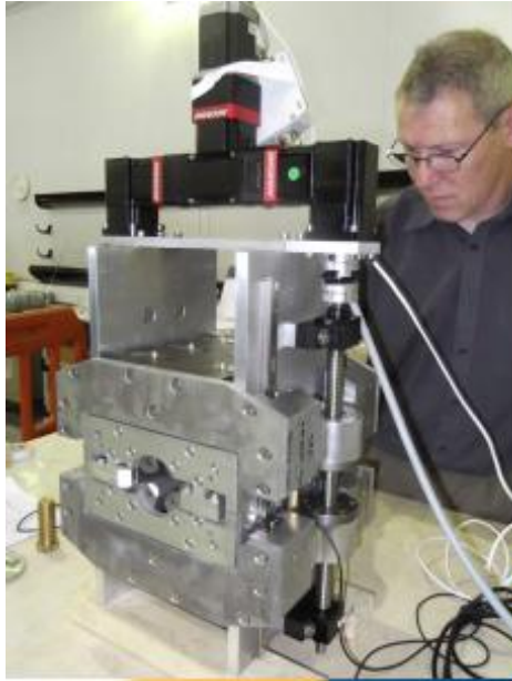
Tunable high-gradient permanent magnet quadrupoles
