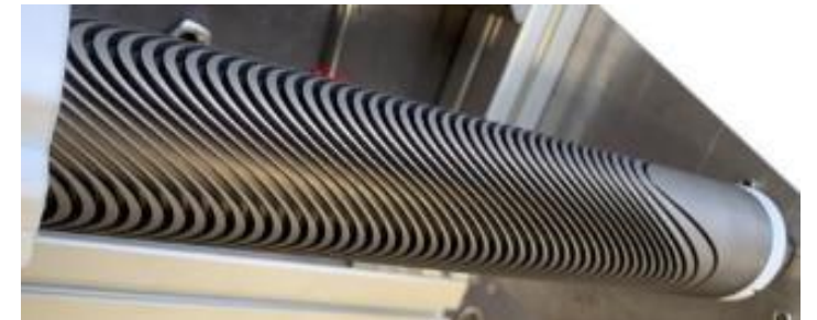
Solution for curved and straight CCT coils combining dipole and quadrupole in the same winding - Courtesy G. Kirby and J. van Nugteren, CERN
