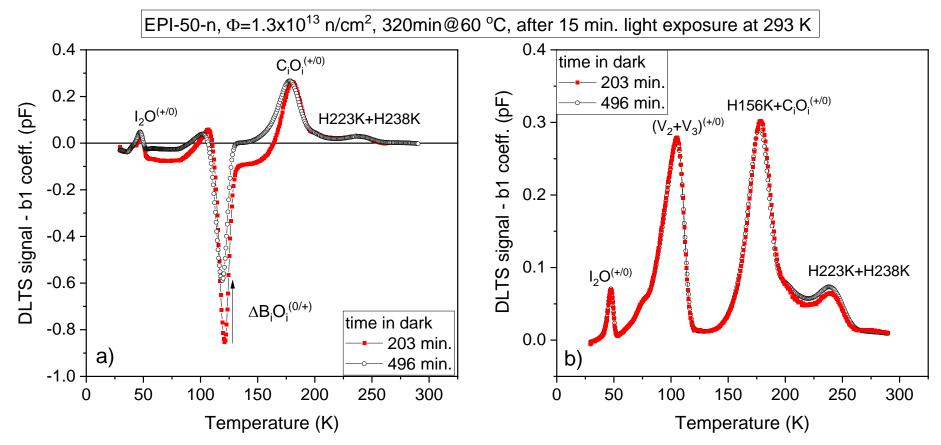
DLTS spectra on irradiated EPI-50 diode recorded after exposing the sample to the ambiental laboratory light at 293K, corresponding to different storage times in dark, for: a) electrons&holes traps (1 V forward bias pulses); b) majority carriers (0 V filling pulses).\*
