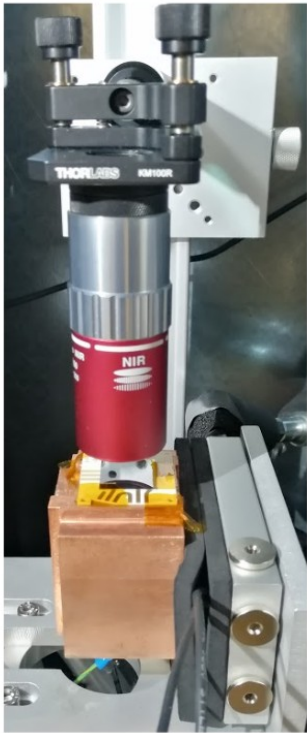
Chip fixed to dummy PCB, backside illuminated ( \lambda = 1.550 \mu\text{m} ) through the \times 100 objective and imaged using an IR camera
