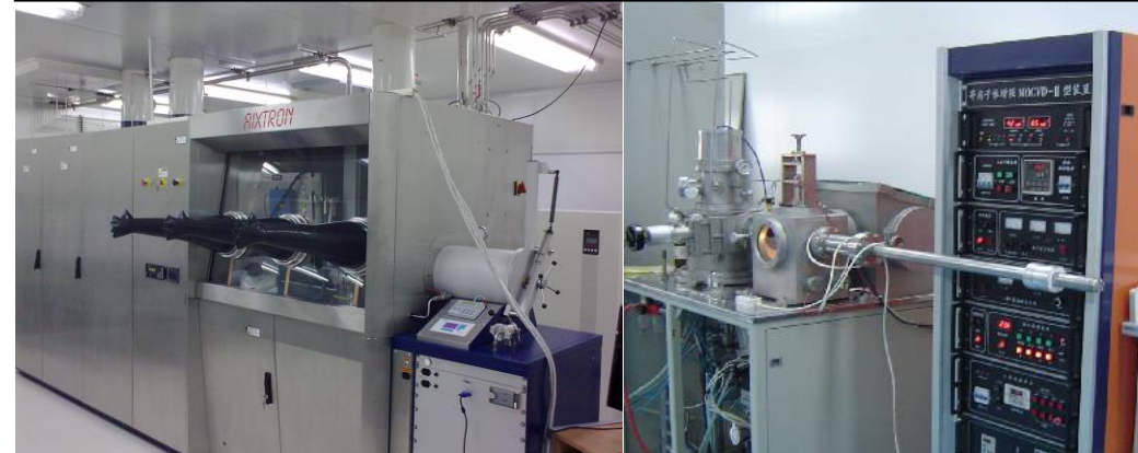
MOCVD growth equipment for nitrides and oxides
