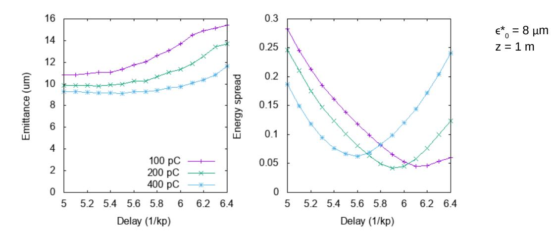
Increasing charge reduces emittance growth ... but increases energy spread
