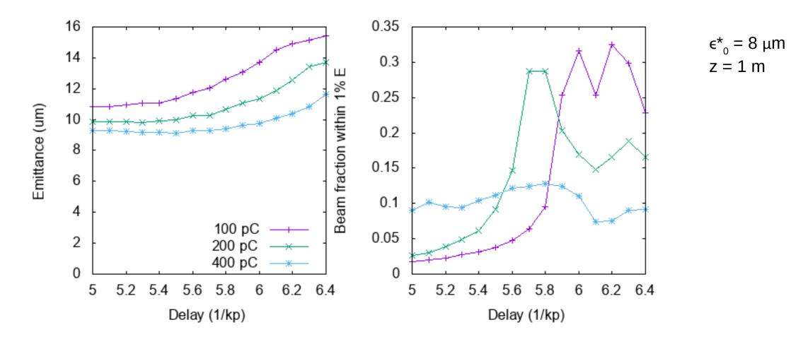
Fraction of beam within 1% energy spread decreases drastically for high charge
