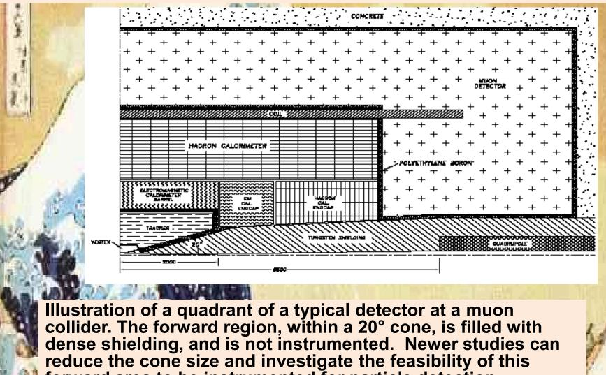
forward area to be instrumented for particle detection.
