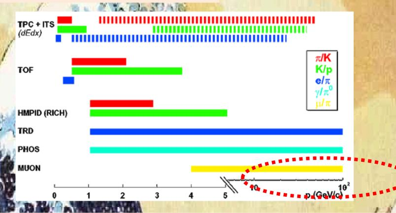
The ability to distinguish electrons from muons can discriminate certain SUSY events from background Run in less than optimized mode for partial particle ID in forward cone
