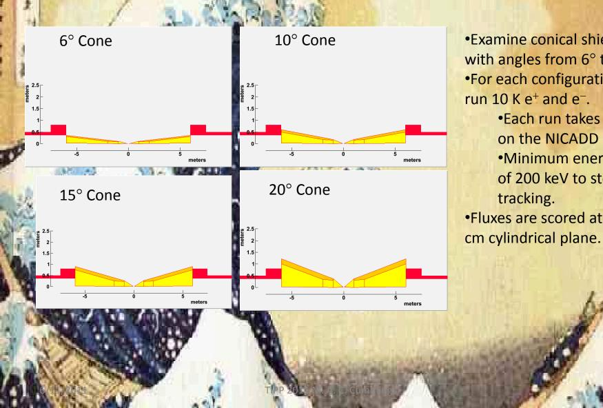
Examine conical shielding with angles from 6° to 20° •For each configuration we run 10 K e<sup>+</sup> and e<sup>-</sup>.
