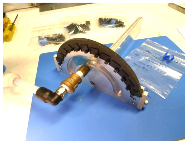
Layer 2 barrel mount on assembly jig
