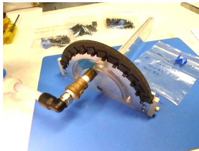
Layer 2 barrel mount on assembly jig
