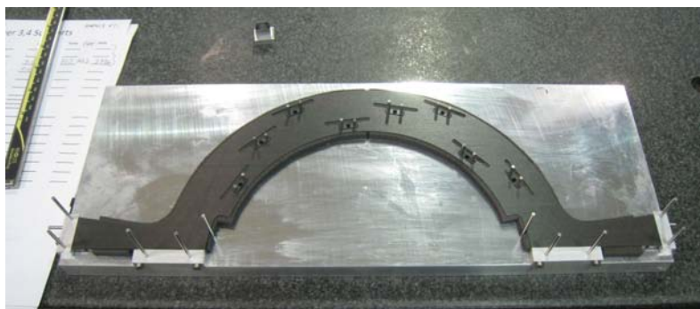
Layer 4 barrel mount on assembly jig
