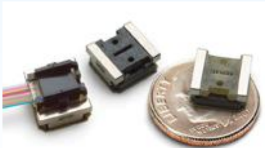
Parallel Optical Engine Tx/Rx (12 channels, 10.3 Gbps/channel)
