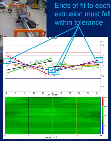
Flatness measurement made for each cell at 5 locations along length of module
