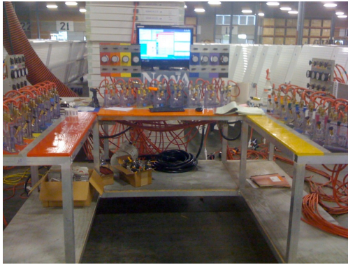
Fig. 8. A 32-channel leak tester is shown. The device measures leaks by counting bubbles as air flows from the reference module (not shown) to the test module.
