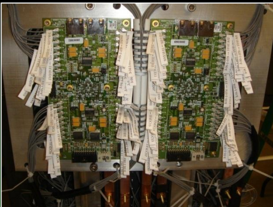
2 TFBs mounted on ECAL super-P0Dule
