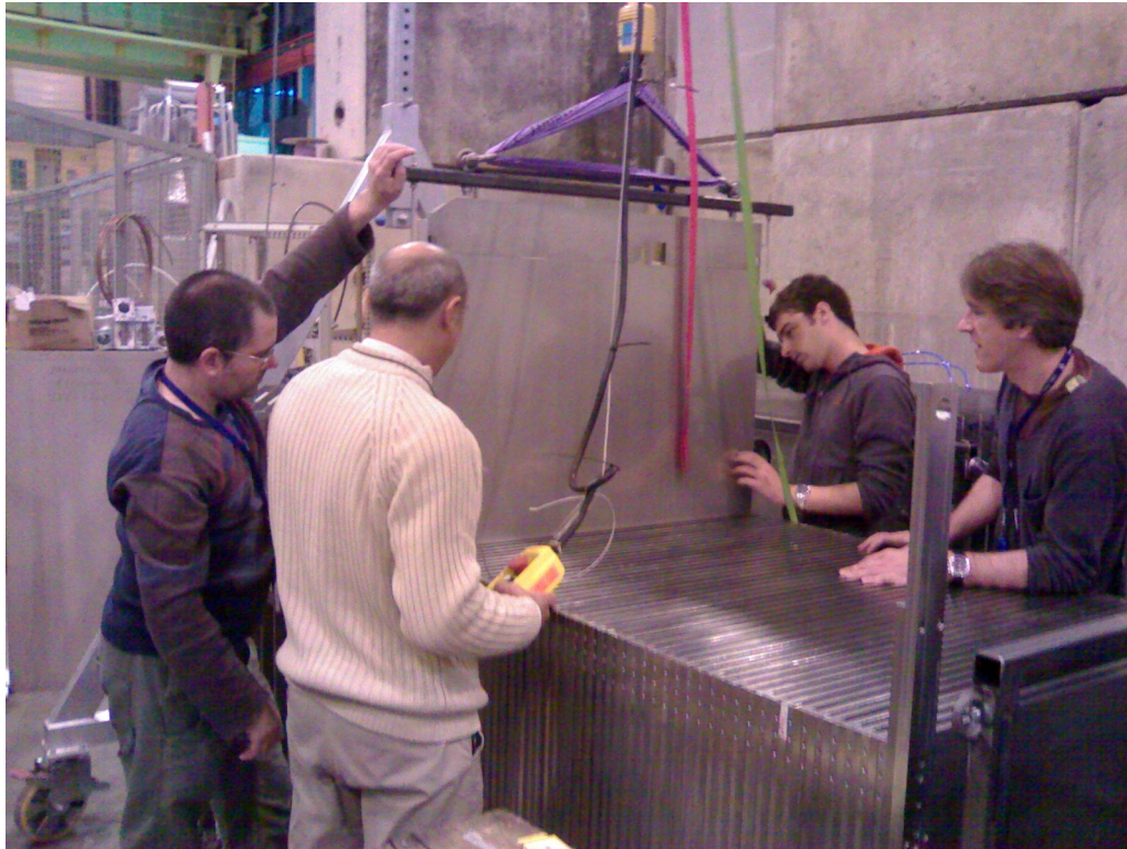
Cassettes insertion in the mechanical structure at CERN
