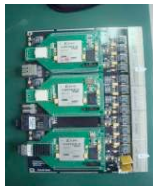
Front-end electronics (ASIC) and 32-Chanel digital board
