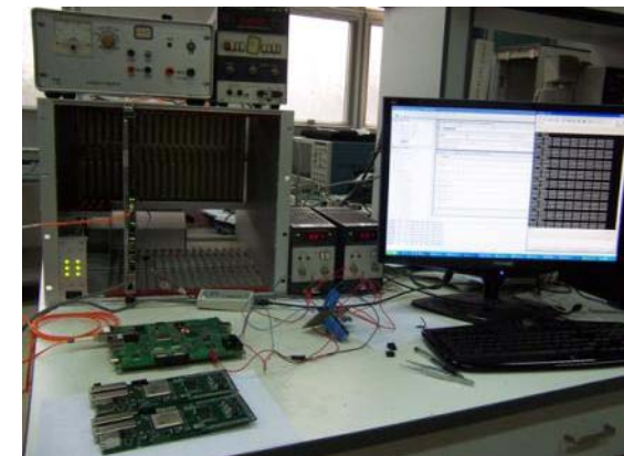
COPPER plugged in VME crate with a File server 14
