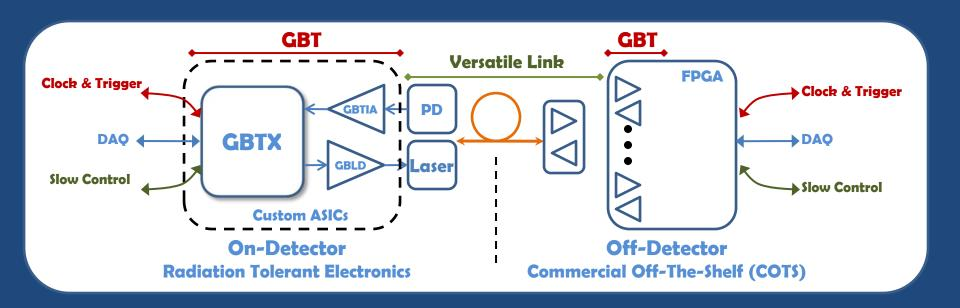
Sister project: Versatile Link to develop optoelectronic components (see Xiang)
