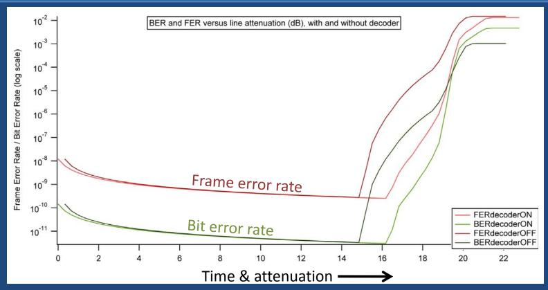
In transceiver mode => transmitting using recovered clock BERT < 9 x 10<sup>-16</sup> (time limited!)
