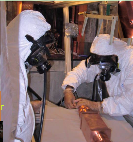
installing DAMA/LIBRA detectors
