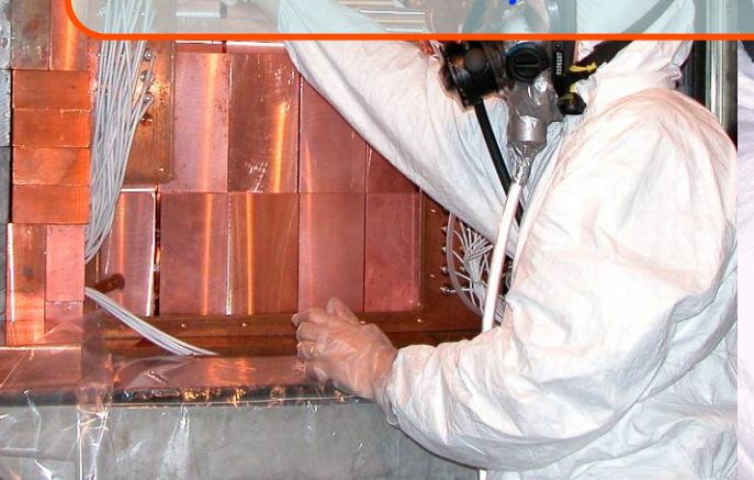
closing the Cu box housing the detectors
