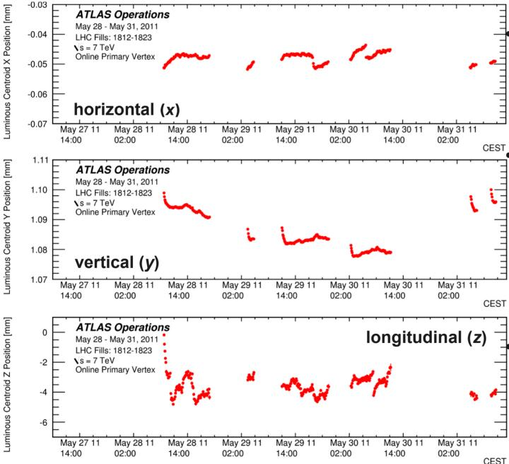
Three-dimensional centroid position is measured over the course of several LHC fills Significant variations of the transverse position (from orbit corrections and drifts) are visible within a fill and from fill to fill Similar significant longitudinal time variations are related to RF-
