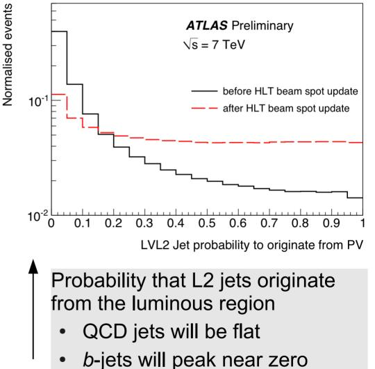
• An off-set beam spot will fake large impact parameters
