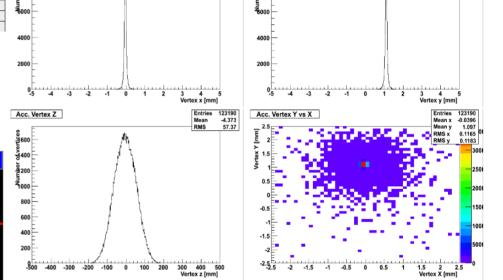
The luminous region parameters are extracted through fits also once a minute
