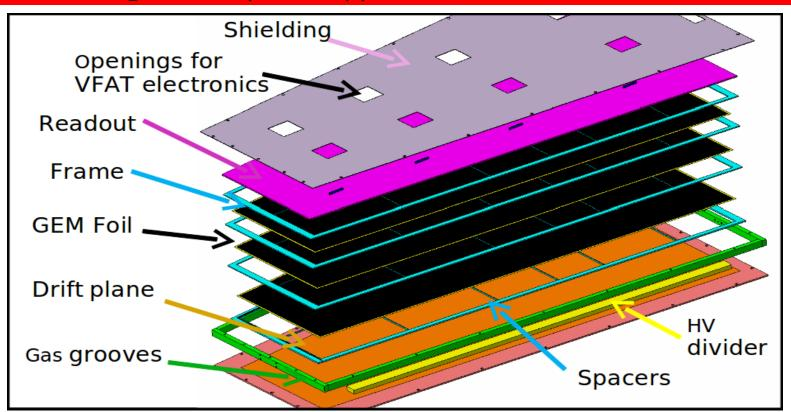
trapezoidal geometry, 990mm × (220 – 455) mm single mask GEM foils, readout 0.8 – 1.6 mm strip pitch \* D. Abbaneo et al., 2010 IEEE Nucl. Sci. Symp. Conf. Rec. 1909-1913; arXiv:1012.1524v2 [physics.ins-det]
