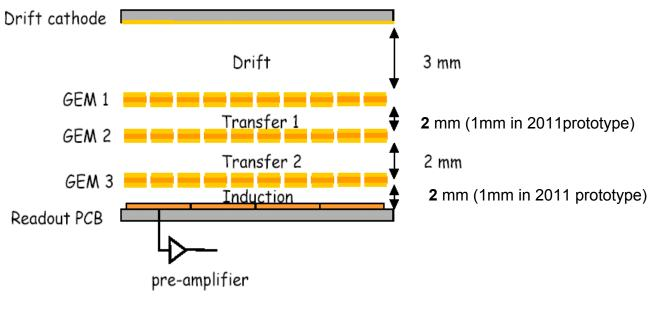
Gas mixture: Ar/CO2 (70/30) Gas flow: ~ 5 l/h
