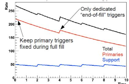
Rates adjusted during the fill with "prescale sets", deployed during a run without the need for a stop/re-start.
