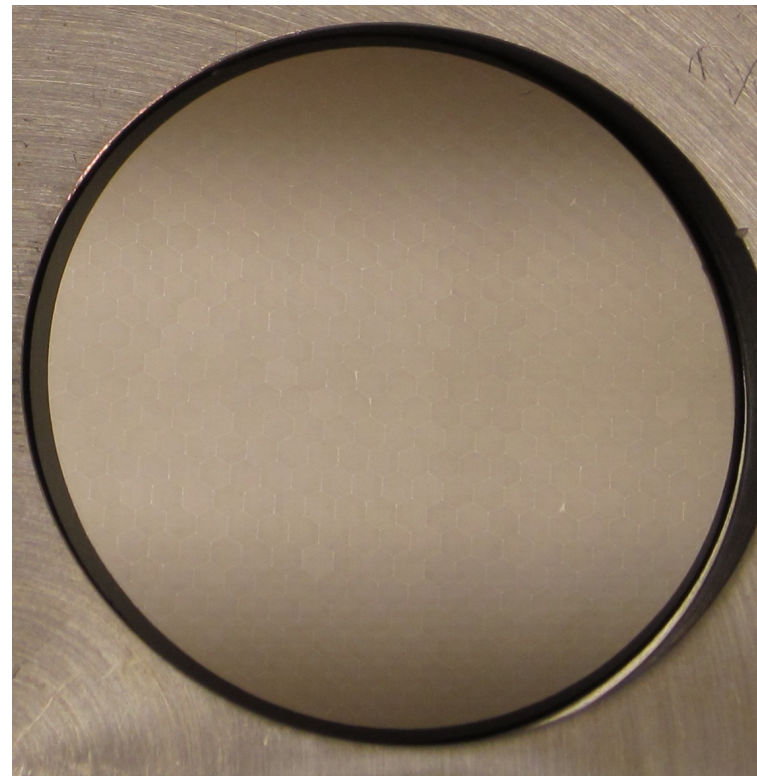
Surface photo for a 20 \mu\text{m} pore borosilicate microcapillary ALD MCP with NiCr electrode .
