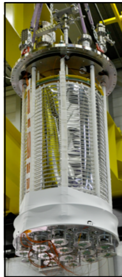
ArDM @ CERN --> LSC (~1t LAr; Greinacher HV- Devise, large area readout, purification, ...)
