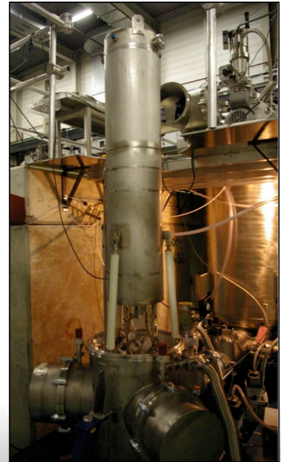
LAr cylinder containing copper cartridge (vacuum insulation removed)
