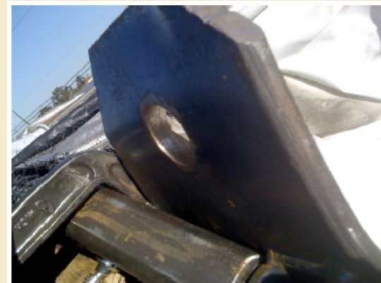
Bent lifting eye on frame
