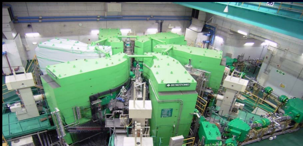
Cyclotron, Osaka University, 1 \mu A, 400 MeV (400W)
