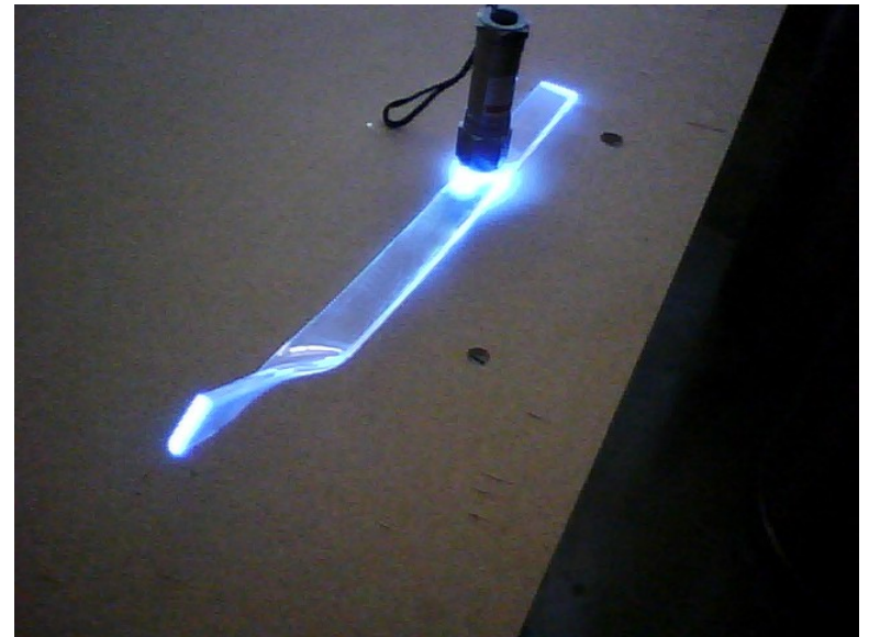
Adiabatic bending still allows light to be transmitted down the rod
