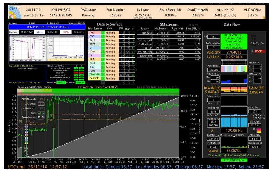
LHC fill 1526: 114 bunch colliding, lumi: L=~3e25/cm^2/s, L1 250 Hz, stream A 116Hz
