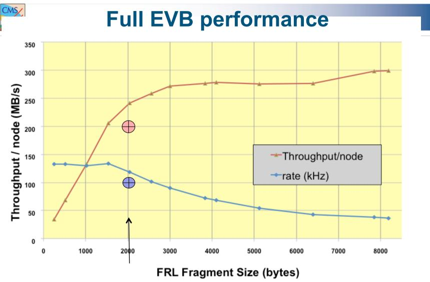
Working point is 2 kByte fragment Rate ~125 kHz, Throughput ~250 MByte/s on each node Aggregate EVB Throughput 125 GByte/s
