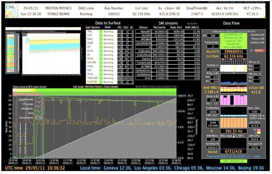
LHC Fill 1815 1092 bunches, 1042 colliding, lumi ~1300 10^30, L1 70 kHz, Stream A ~400 Hz, HLT CPU ~50%
