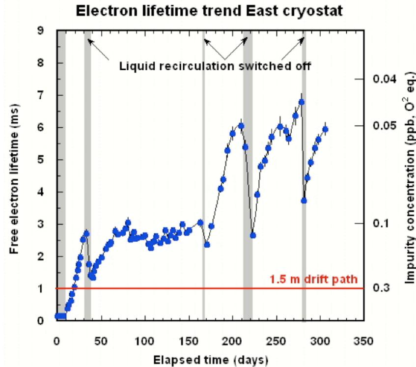
Simple model: uniform distribution of the impurities, including internal degassing, decreasing in time, constant external leak and liquid purification by recirculation.
