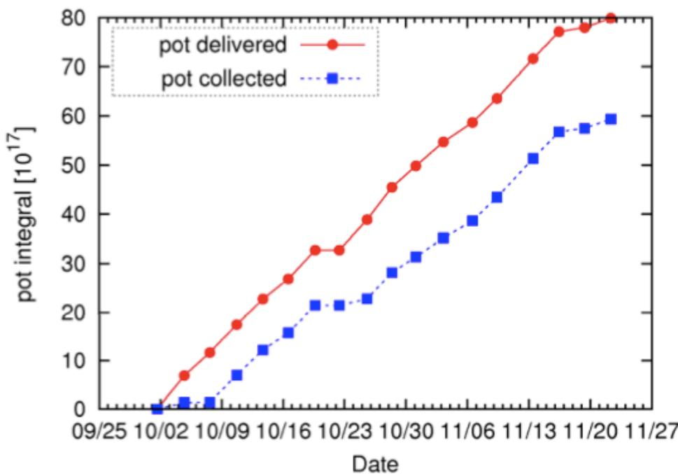
Number of collected interactions compared with number of interactions predicted ((2.6 v CC + 0.86 v NC)  $10^{-17}$ /pot), in the whole energy range up to 100 GeV, corrected by fiducial volume (424 t) and DAQ dead-time.
