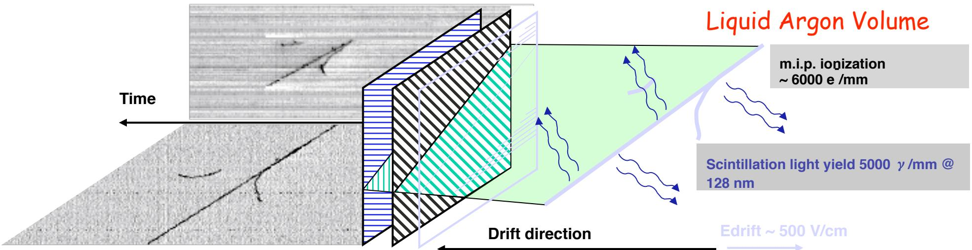
Electrons from ionizing track are drifted in LAr by  $E_{\text{drift}}$ . They traverse transparent wire arrays oriented in different directions where induction signals are recorded. Finally electron charge is collected by collection plane.
