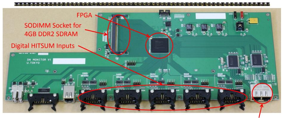
A prototype of the new DAQ module was made.
