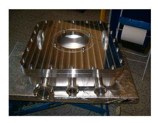
The prototype was tested under vacuum
