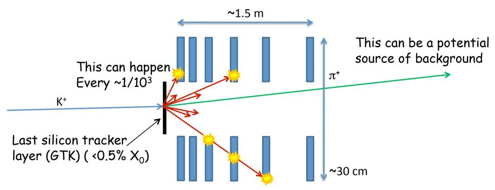
Inelastic interactions can be identified detecting the large angle products using a set of "guard rings"
