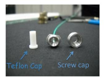
A Teflon cap define the reference plane for the fiber It used to protect the polished side of the fiber during transport and handling.
