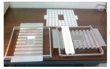
Bars are precisely glued together using a custom reference jig
