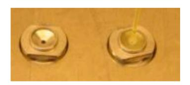
A 50  $\mu$ m tolerance in the fiber-SiPM coupling is reached
