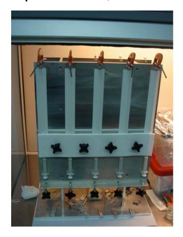
The glue is injected from the bottom using a syringe to reduce the probability to produce air bubbles.
