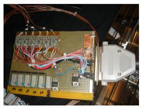
20 X fast amplifiers & Individual-adjustable SiPM bias voltage: O(mV) resolution 0.1% stability
