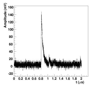
Fast 20X amplification after 1.5 m coaxial cable
