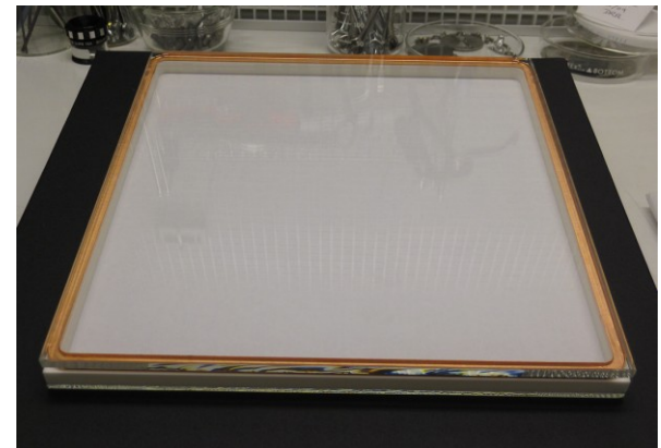
Ceramic body of the proposed photodetector
