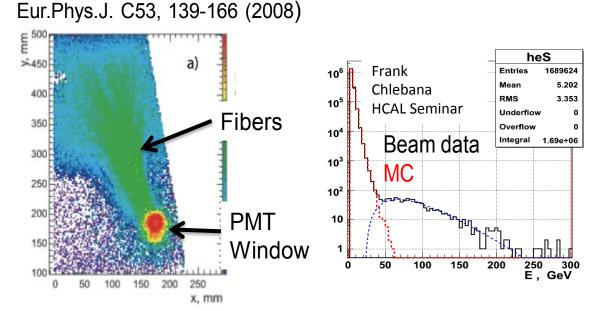
Previous CMS Simulation has a problem to simulate HF Noise because it killed particles immediately when they entered detectors.
