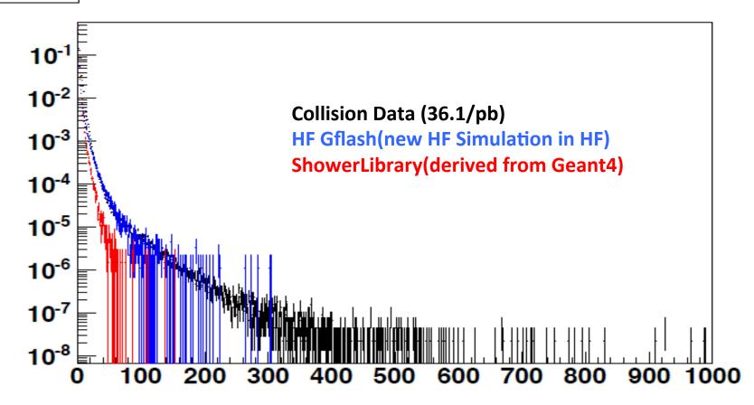
HF Gflash has better agreement to 36.1 pb-1 Certified Collision Data compared to previous simulation
