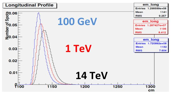
Geant4 will need days to simulate the shower profile of 1 TeV electron gun. Fortunately HF Gflash only need few seconds to simulate the interaction of very high energy particles with detector and gives good longitudinal profiles for very high energy particles(higher than 1 TeV)
