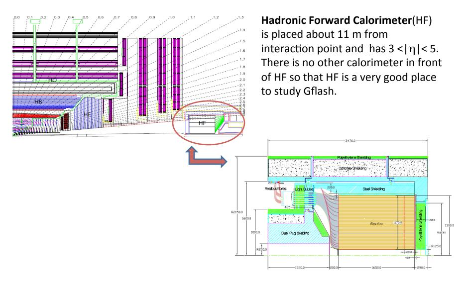
HF has **Long** and **Short** Fibers to differentiate shower from electromagnetic & hadronic particles
