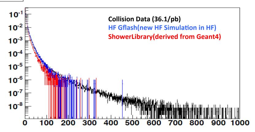
HF Gflash has better agreement to 36.1 pb-1 Collision Data compared to previous simulation
