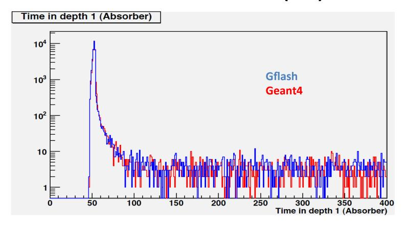
HF Gflash can perform timing simulation from interaction point(IP) to PMT very well with less electricity consumption
