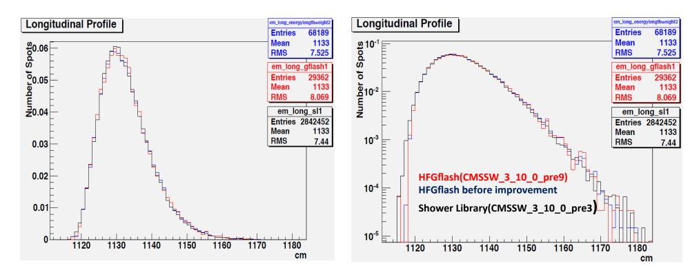
Longitudinal profile produced by 100-GeV electron gun using HFGflash, old HFGflash and Shower Library(based on Geant4)
