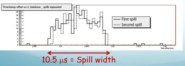
The precision of this prediction is ~20  $\mu$ s >> jitter of local clock (GPS based). Still enough for triggering purpose.
