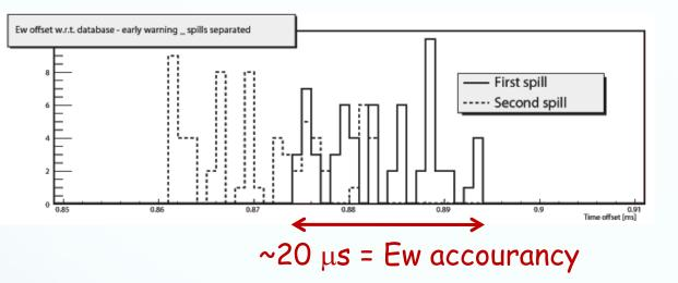
An "early warning" (Ew) message is sent from CERN to LNGS 150 ms before each extraction. This message contains the predicted extraction time.
