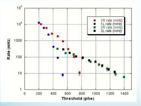
Dark count rates allow a minimum threshold of ~1000 phe<sup>-</sup> (HT) for the sum signal of each chamber.
