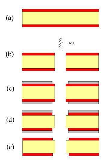
Copper 20µm FR4 160µm Thickness 200µm Hole 200µm pitch 500µm
