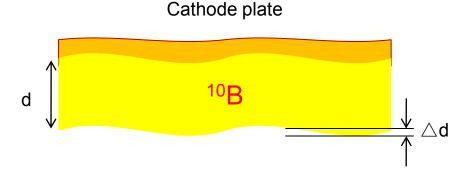
$d \to 0, \ \eta(x, y) = d(x, y) \int S(E, x, y) n \sigma(E) dE$ Uniform S(E):
