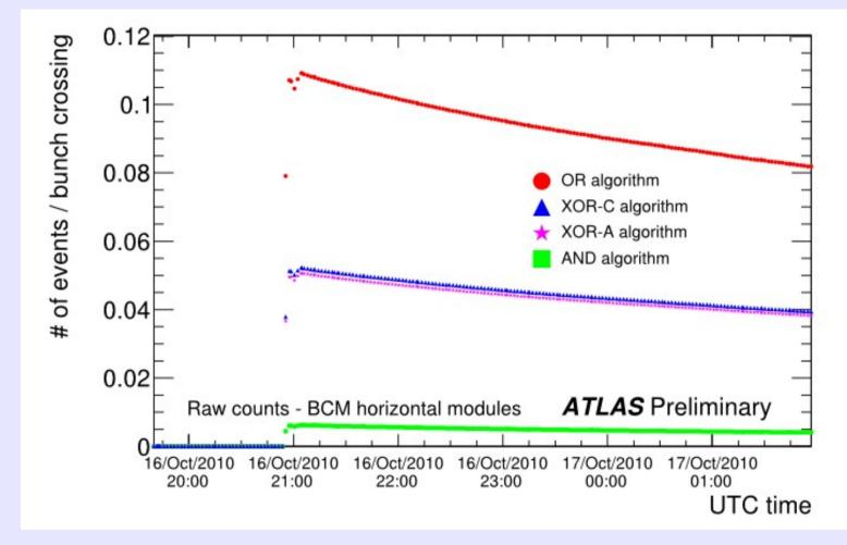
Four algorithms with different coincidence criteria between sides A and C.
