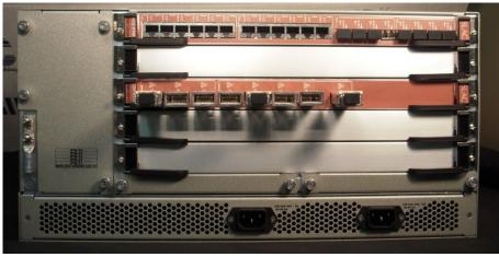
Phase 1 RCE and CI boards are in use at Linac Coherent Light Source
