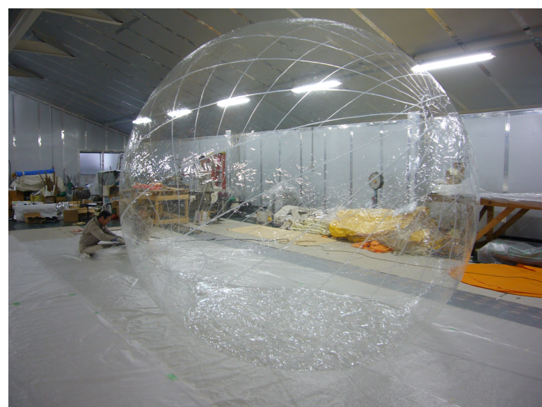
Mini-balloon fabrication with 25 \mu m Nylon film
