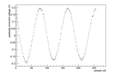
Visible attenuation along chip input at higher frequencies
