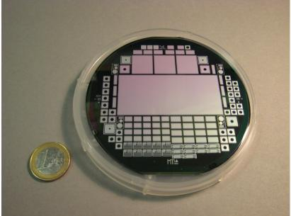
Flip-chip bonding for prototypes done at IZM (Berlin, Germany) in 2010 Target read-out wafer thickness is <100 µm for final production
