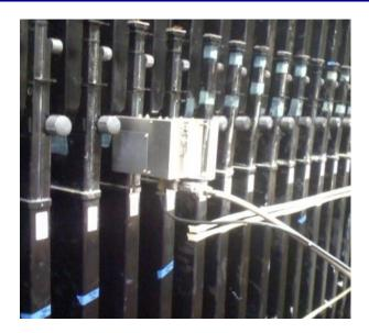
•NDOS: Experience qualifying scintillator. Refined filling procedure for record keeping and cleanliness. Found internal obstructions preventing complete fills.
