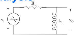
$$v_{i}(t) = V_{p} \cos(\omega_{O} t)$$
