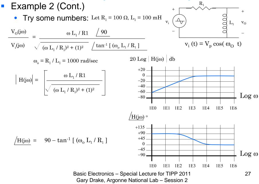
Example 2 (Cont.) +00000 **Examining Bode Plots for features** Vi v<sub>0</sub>  $L_1$  $V_0(j\omega)$ 90  $\omega L_1 / R1$  $/ an^{\cdot 1}$  [ ( $\omega_{
