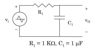
$$V_{O}(j\omega) = \frac{V_{i}(j\omega)}{\sqrt{(\omega_{o} R_{1} C_{1})^{2} + 1}} / \frac{-\tan^{-1} [(\omega_{o} R_{1} C_{1})]}{\sqrt{(\omega_{o} R_{1} C_{1})^{2} + 1}} \Rightarrow Phasor Form$$
