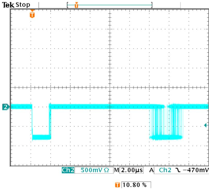
Pulses with 150nA input current
