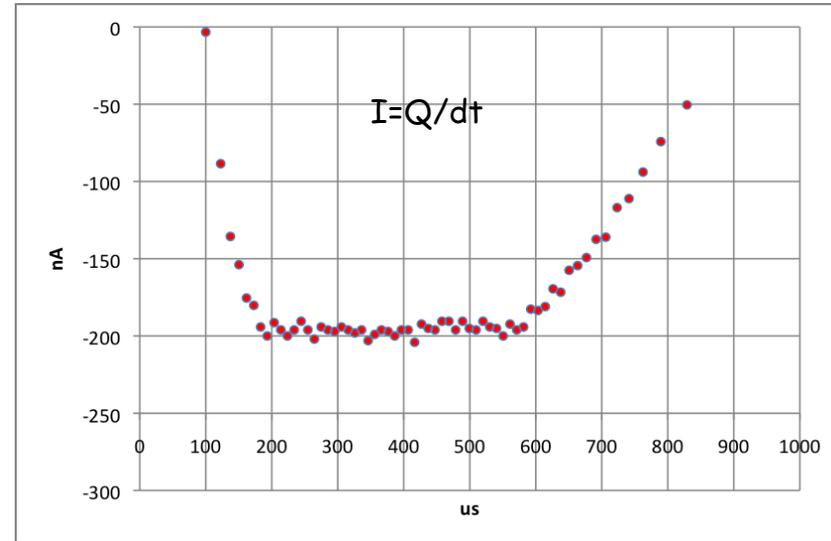
FPGA-TDC data generated by measuring time between pulses
