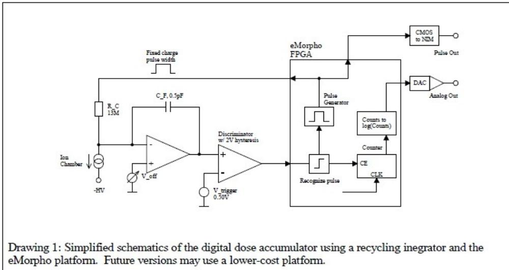
Drawing 1: Simplified schematics of the digital dose accumulator using a recycling integrator and the eMorpho platform. Future versions may use a lower-cost platform.
