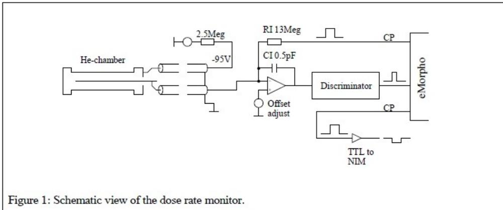
Figure 1: Schematic view of the dose rate monitor.
