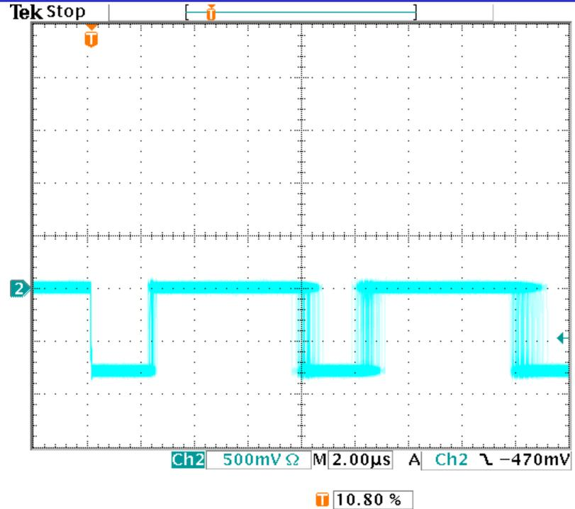
Pulses with 300nA input current
