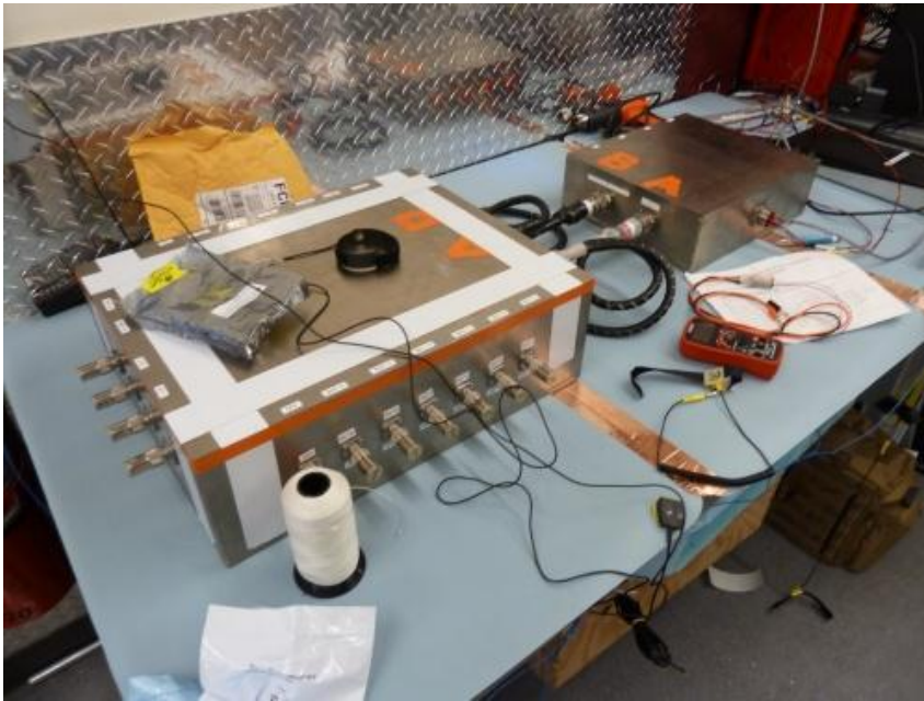
Testbed electronics plus DC-DC converter box
